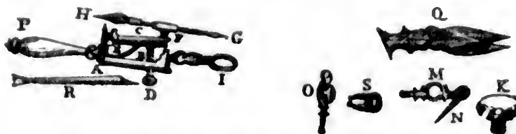
LIEBERKÜHN'S SIMPLE MICROSCOPE (1741).
