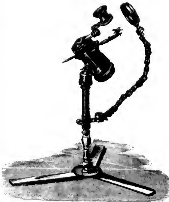
CULPEPER'S SIMPLE MICROSCOPE (WILSON'S FORM, ante 1738?).
