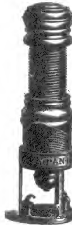
CAMPA NI'S COMPOUND MICROSCOPE (ante 1665?).
