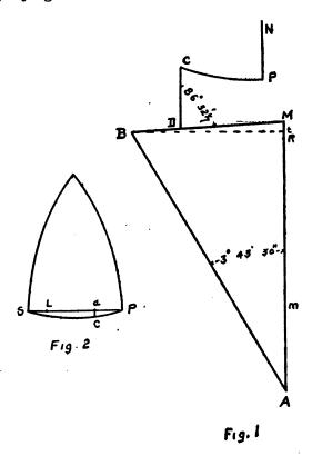
in running out the boundaries. NP is a true meridian, PC an arc of a parallel, CD a portion of a true meridian, MDB a straight line making an angle of 86° 32½ with CD, and BA a line connecting with the terminal point A and making an angle of 3° 43′ 30″ with the direction of the true meridian.
